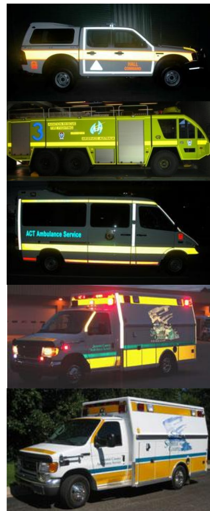
Figure 9 – Examples of different contour markings. Note the contour stripe color matches the body color and is therefore invisible in daylight.
